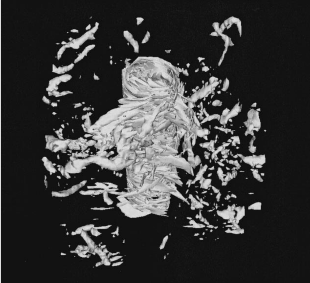
FIGURE 2. Iso-vorticity surfaces at |\omega| = \omega_s , in turbulence around a vortex filament of strength \Gamma = \pi/2 calculated by RDT: (a) initial state t = 0 , \omega_s = 8.85 and (b) after half a revolution t = \pi , \omega_s = 30.65 . Note that u_0 \approx 0.8 , L_x \approx 1.2 so \omega_x \approx 10u_0/L_x at t = 0 .
